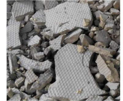
过滤后滤饼含水率45%-60% Moisture content of filter cake 45-60%
